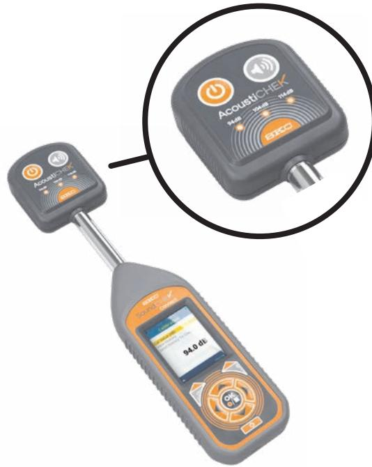
Introducing the SKC AcoustiCHEK Calibrator! AcoustiCHEK is specifically designed to provide easy and accurate calibration for the SKC NoiseCHEK Dosimeter, SoundCHEK Essential Sound Level Meter, and SoundCHEK Connect Sound Level Meters. In the lab or in the field, AcoustiCHEK is there for your noise and sound level meter calibration needs and backed by SKC's high-level quality and expertise.
